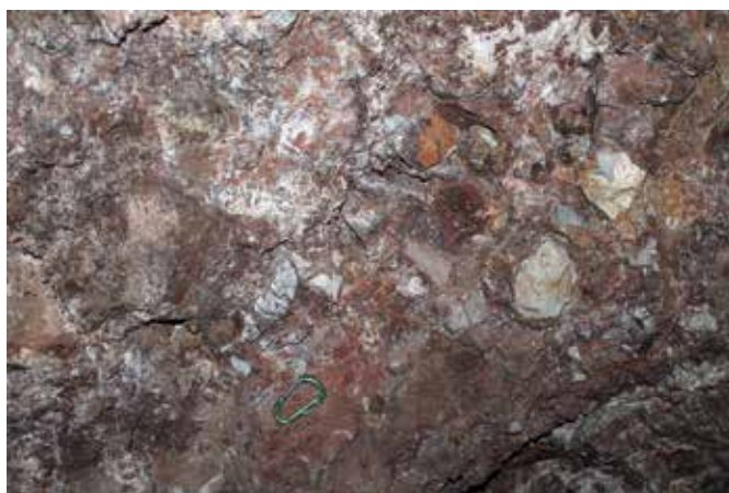
Figure 4: Limited argillic alteration located 10 meters from the main vein outcrop. The white mineral is kaolinite, red minerals are hematite and unknown iron oxy-hydroxides. Clasts are brecciated andesite, dacite, and rhyolite. Sericite and chlorite are visible with a hand lens. Field of view is 4 feet.
