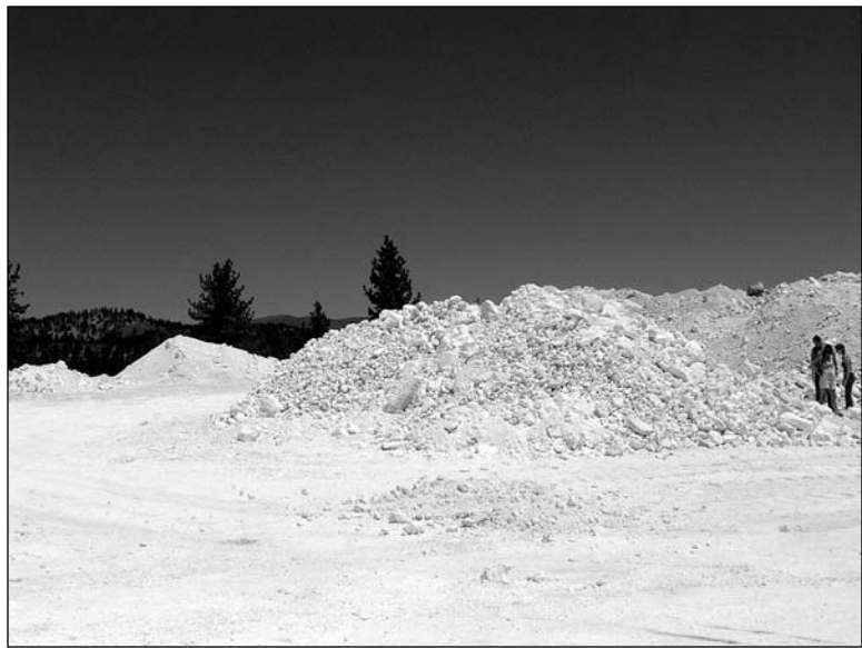
Figure 2-9. Kaolinite “ore” stockpile at the Huntley Mine open pit. [D. R. Jessey photo]
