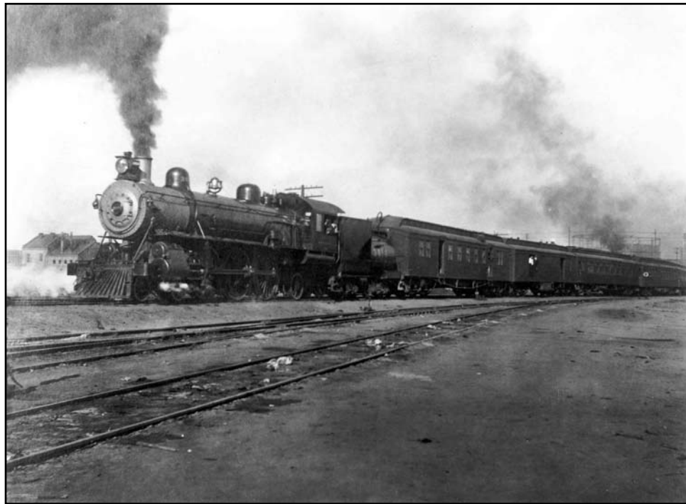
Figure 1. San Pedro, Los Angeles & Salt Lake Railroad 4-6-2 Locomotive No. 3414 with a Vanderbilt tender pulls out with a passenger train which will cross the lands now in Mojave National Preserve, early in the history of the railroad. The train may be the crack "Los Angeles Limited."
