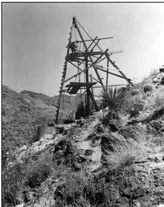
Test drilling on the east orebody at the Vulcan Mine. Photograph from the Bud Davenport collection, Mojave National Preserve.
