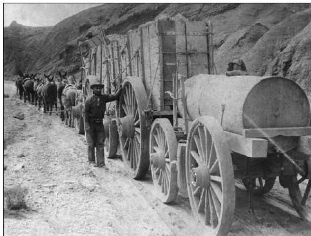
Figure 6. Borax ore in wagons. The empty water wagon was hauled from Borate for refilling. Ed Pitcher, teamster, standing.
