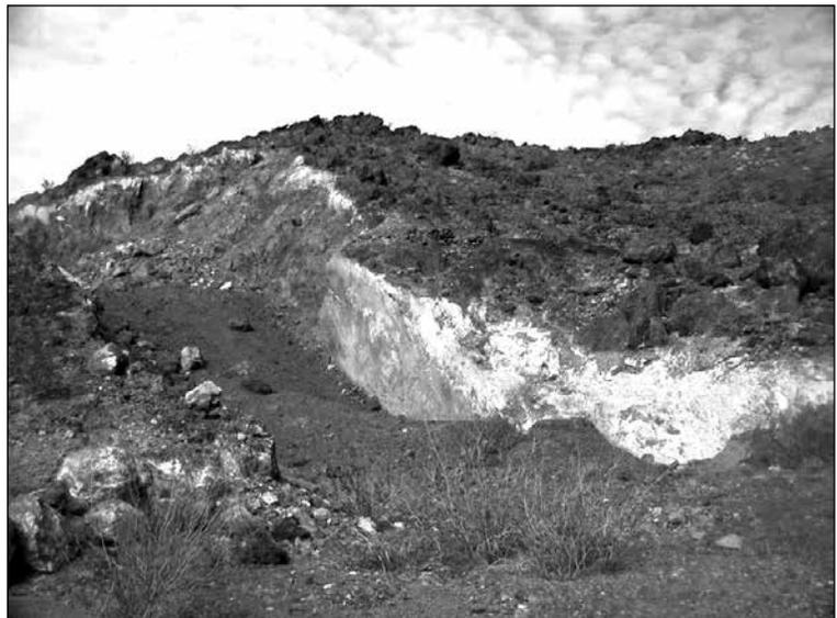
Figure 8. Black Butte Mine northwest trending fault with barium and manganese oxides.
