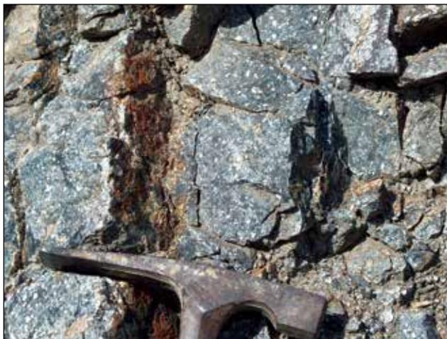
Figure 12. View of metavolcanic rock exposed in the north wall of the open pit mine. Note the light colored plagioclase grains within the dark fine-grained matrix. Also note the near vertical mineralized zone under the rock hammer head and just left of the handle.
